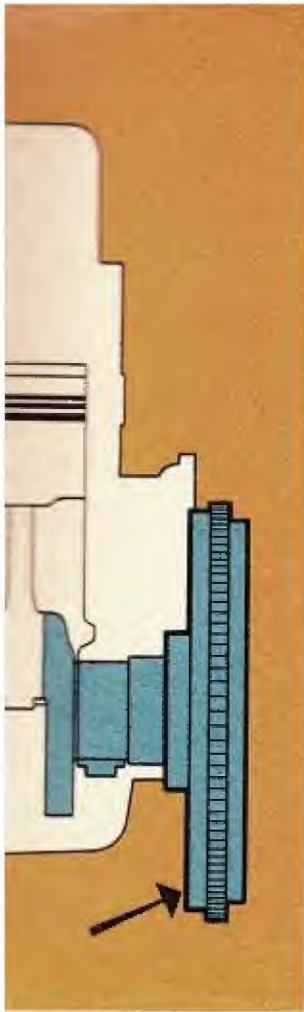
Motor vehicle engines use the 'inertia' of a revolving flywheel to smooth irregularities in power strokes.
